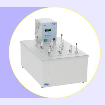
Delivered as complete D3231 apparatus
